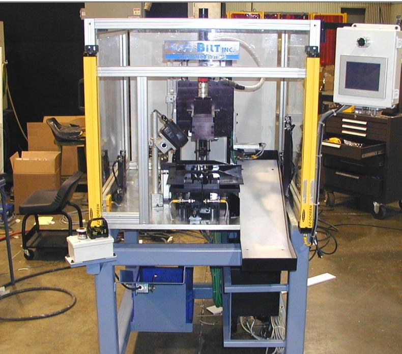
*Torque Testing Machine with Auto Part Eject*
