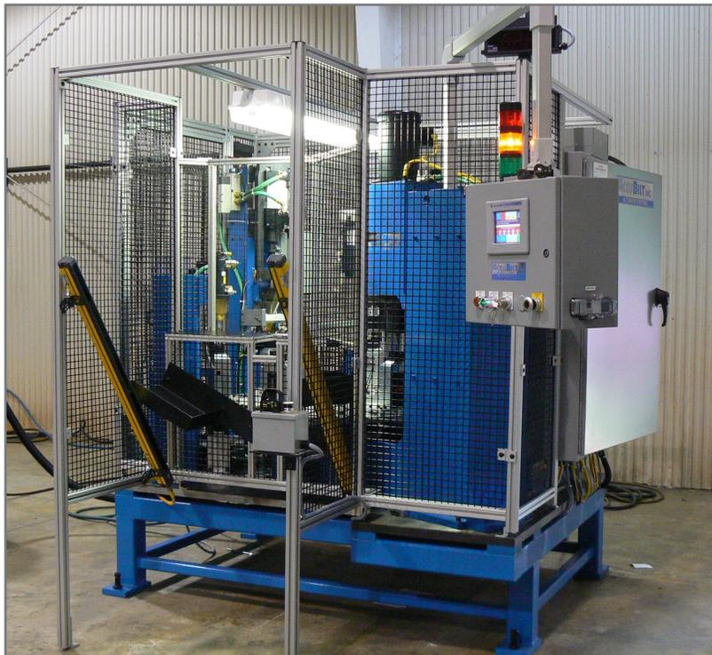
6-Station Indexer with Drill, Pin Feed, Press & Test
