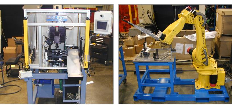
Torque Testing Machine with Auto Part Eject
