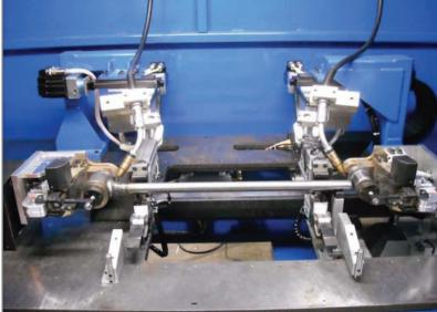
Lathe Welder setup for welding axles and other small diameter parts
